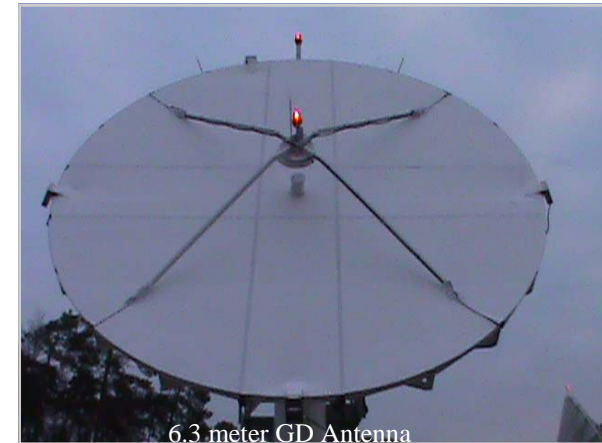
6.3 meter GD Antenna
